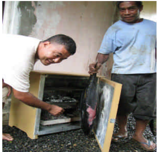
Robert Andreas here points to the energy-efficient charcoal oven. Alpret Bernardo looks on, holding a fish to be baked. This oven uses charcoal from coconut shells and hard wood. The oven is energy-efficient compared to open fire cooking, offers a healthy way of cooking (baking has advantages over frying), is convenient (compared to the traditional way of making an umhw, or earth oven), and is money-saving.
